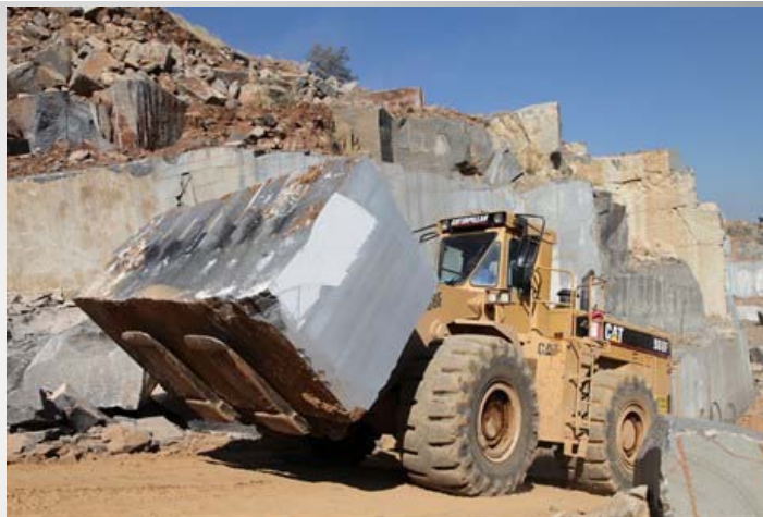
A Cat 988 transports a cut block, weighing up to 20tonnes, from the quarry to the nearby dressing yards on site
